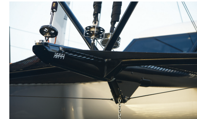
A high-modulus carbon longeron ensures structural stiffness
